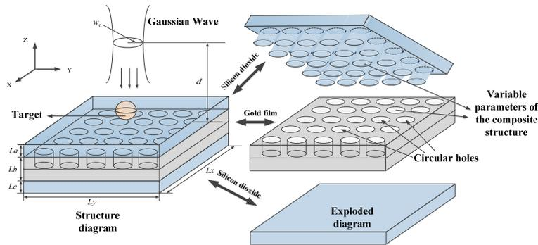
Fig. 1. Schematic of the target placed on the composite metallic film with periodic structure.
